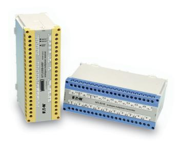
MTL830 range of multiplexers with Modbus<sup>®</sup> outputs provide a cost-effective alternative to single-loop isolation. The cost of installed wiring is reduced by up to 50% by communicating the input of multiple hazardous-area sensors over dual-redundant data highways. Further savings are achieved by reducing the number of inputs to the host, cabinet space and weight.
